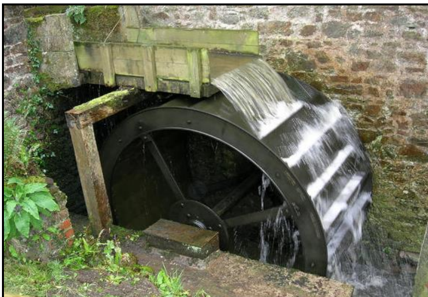
Fig.1 Overshot waterwheel bridge Mill, Bridgerule 51
